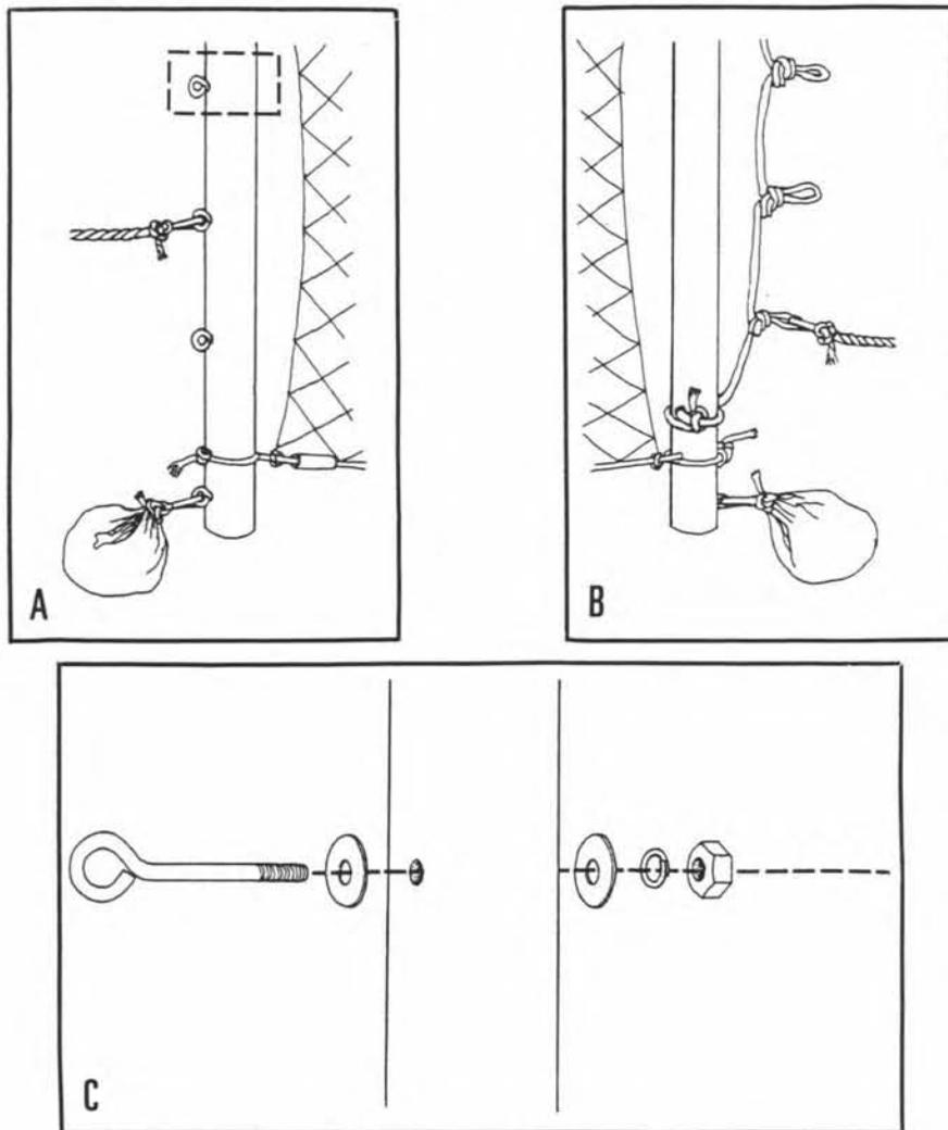
**Figure 1.** Diagrammatic representation of brail modifications for seine towing. A) Brail with eye bolts. B) Brail with knotted rope replacing eye bolts. C) Exploded view of eye bolt attachment. See text for details.
